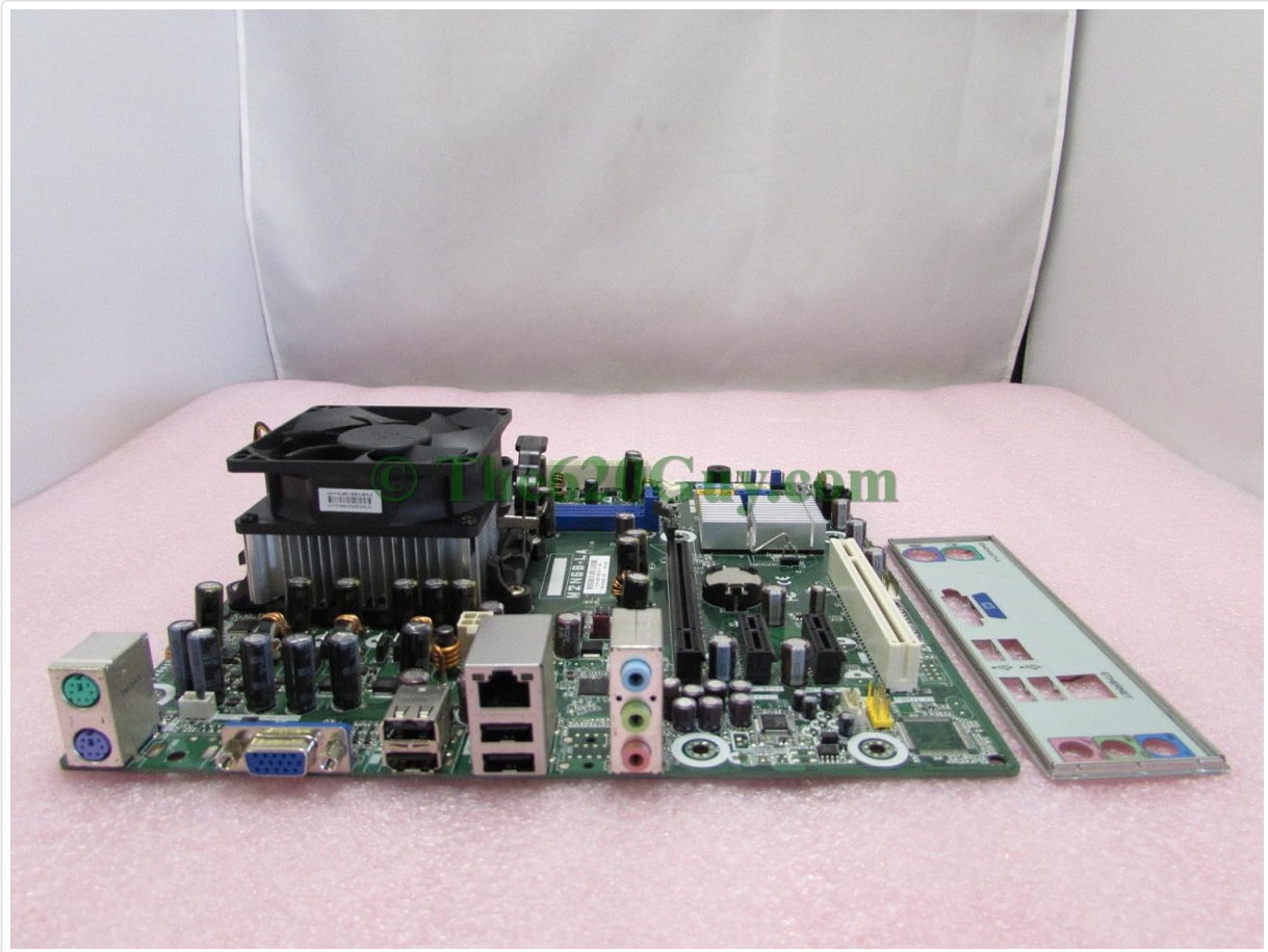
Figure 2.2: Side view of the motherboard, illustrating the CPU heatsink and fan assembly, along with the rear I/O panel.
