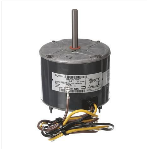
Figure 3.1: Genteq 5KCP39FGU997AS Condenser Fan Motor. This image shows the cylindrical motor body, the shaft extending upwards, and the attached wiring harness with multiple colored wires (yellow, black, brown, and a ground wire) bundled together.
