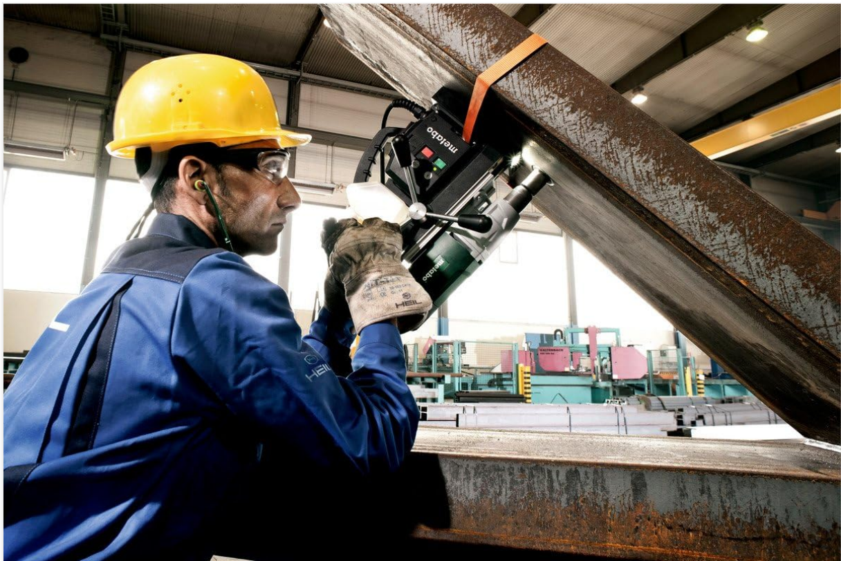
Figure 2: An operator demonstrating the use of the Metabo MAG 32 Electromagnetic Core Drill on a large metal beam, highlighting its capability for overhead and vertical applications.
