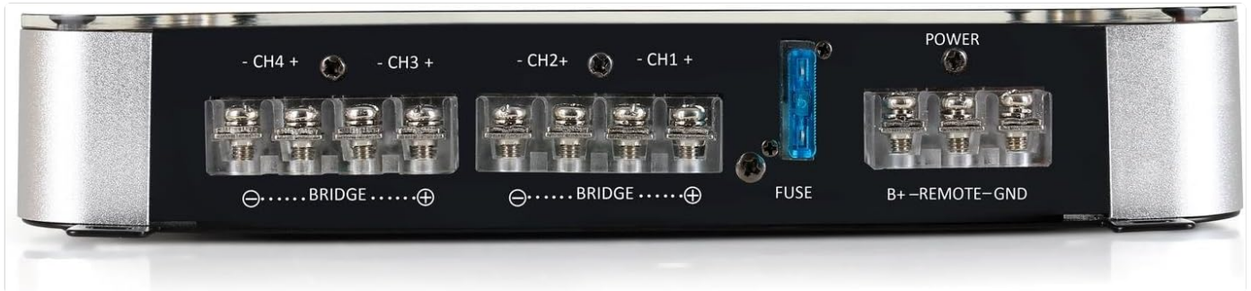
Figure 4.1: Rear panel of the amplifier displaying the power input terminals (B+, REMOTE, GND) and speaker output terminals (CH1+, CH1-, CH2+, CH2-, CH3+, CH3-, CH4+, CH4-), along with the fuse slot.
