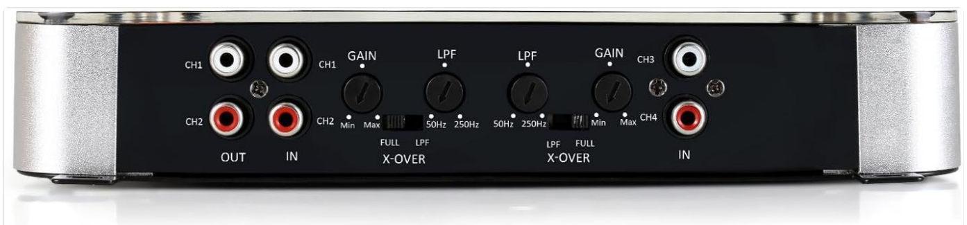
Figure 4.2: Rear panel of the amplifier displaying the RCA input/output jacks (CH1 OUT, CH1 IN, CH2 IN, CH3 IN, CH4 IN) and control knobs for GAIN and LPF/X-OVER settings.
