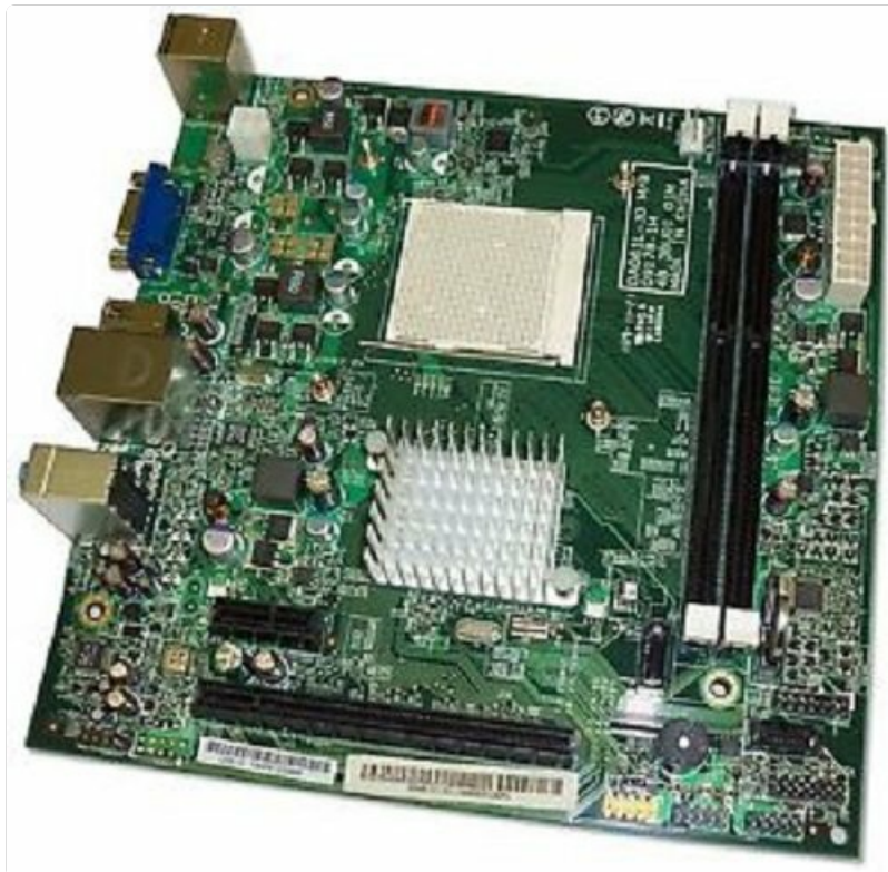
Figure 1: Overview of the eMachines EI1358 (MB.NBT01.001) AM2 Desktop Motherboard. This image displays the top-down view of the motherboard, highlighting its various components such as the CPU socket, RAM slots, PCIe slots, and I/O ports.
