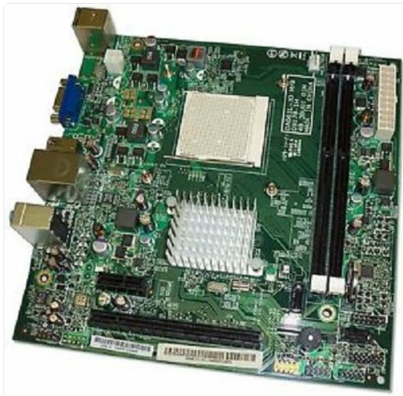
Figure 2: Diagram illustrating key components and connectors on the eMachines EI1358 Motherboard. This includes the CPU socket, DIMM slots, PCIe slots, SATA ports, USB headers, and front panel connectors. Refer to this diagram for component identification during installation.
