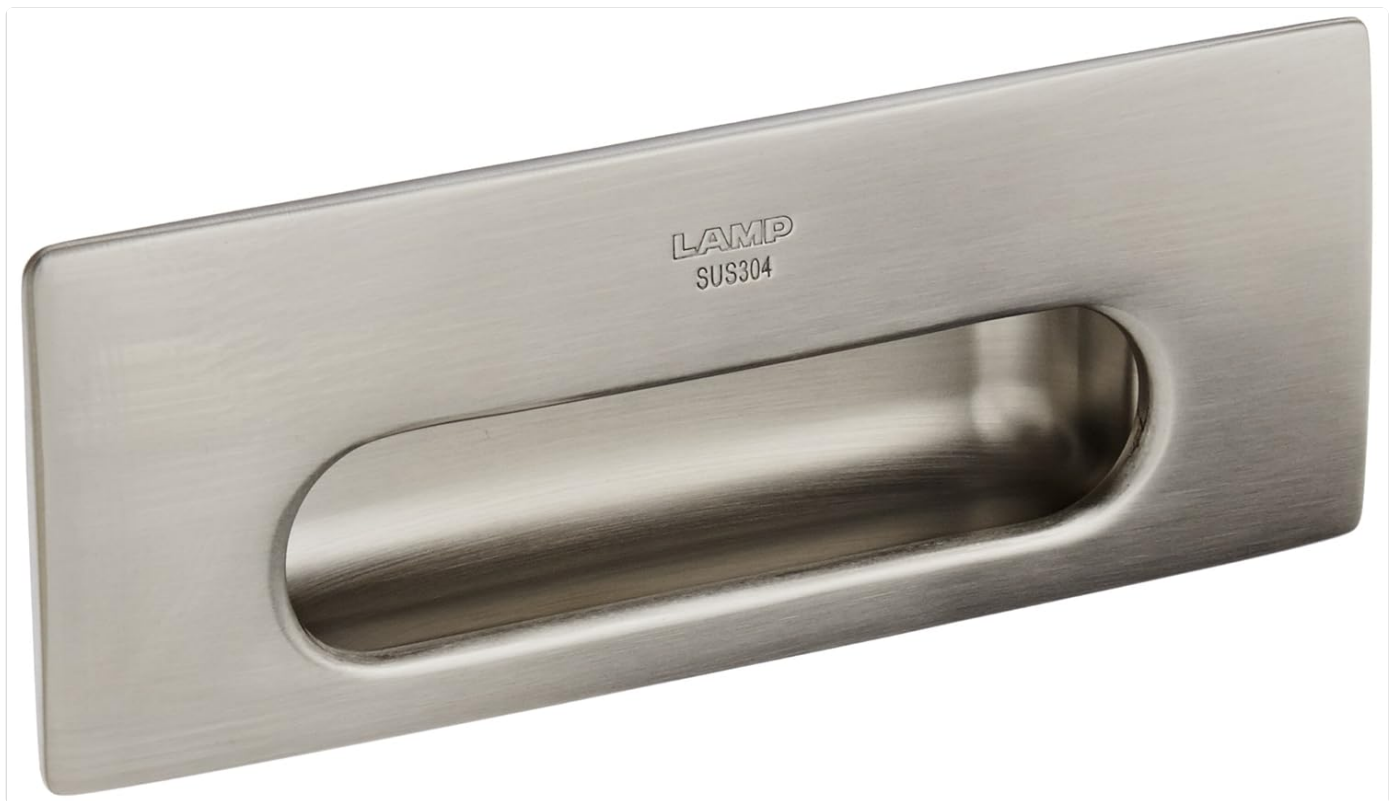
Image 1: The Sugatsune Lamp HH-KL160 Pull, a rectangular recessed handle made of satin-finished 304 stainless steel. The brand "LAMP" and material "SUS304" are subtly engraved on the surface.
