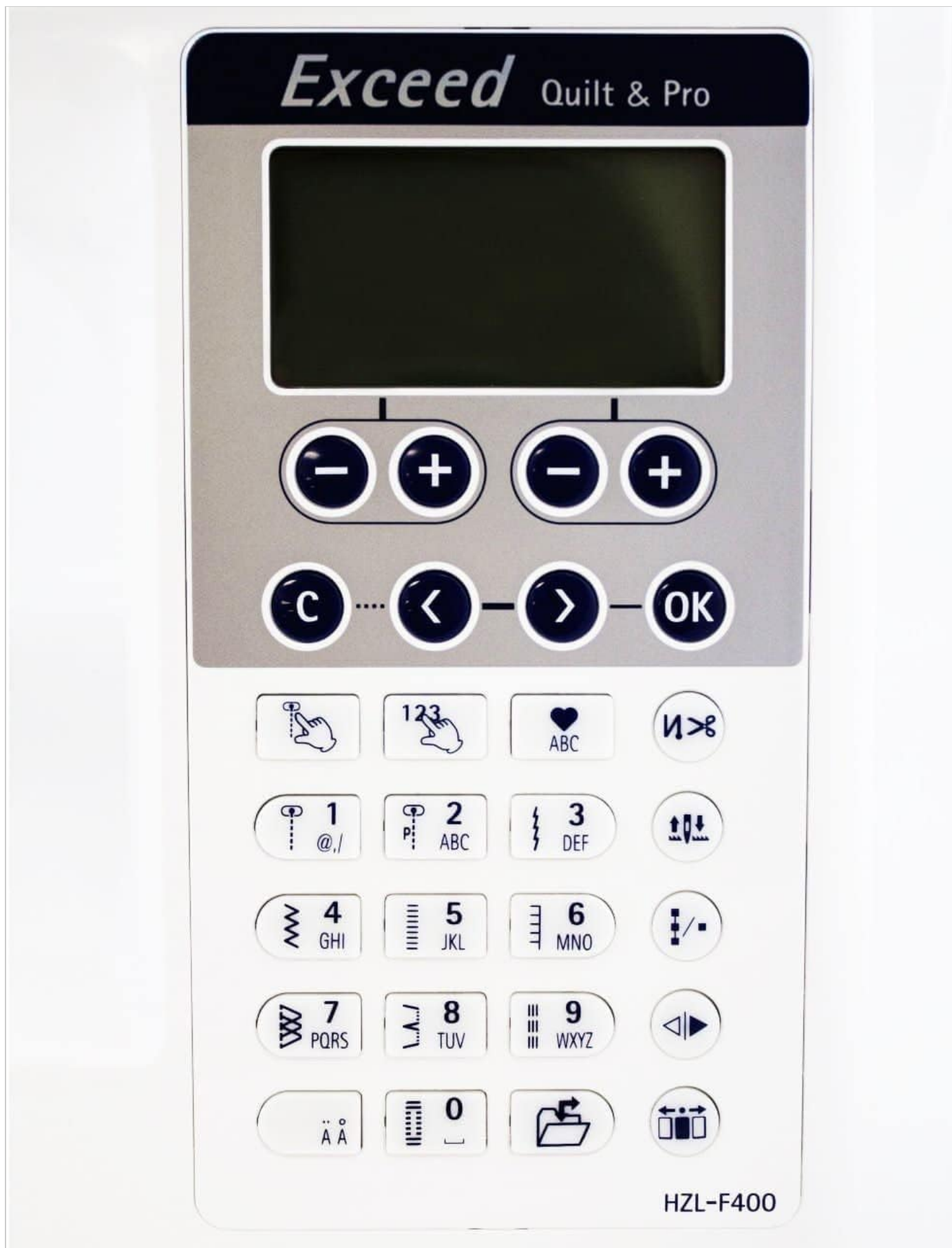
Figure 3.2: Close-up of the Juki HZL-F400 control panel and LCD screen, showing stitch selection buttons and display.
