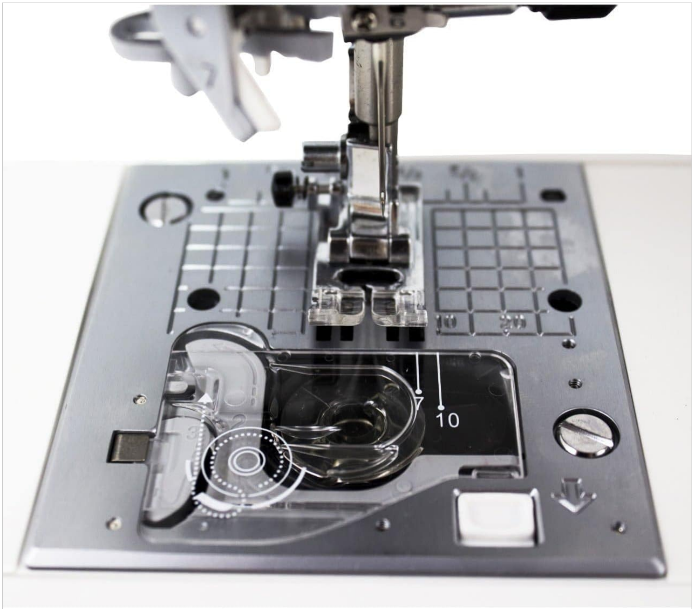
Figure 4.1: View of the Juki HZL-F400's transparent bobbin cover and drop-in bobbin system, showing the bobbin in place.
