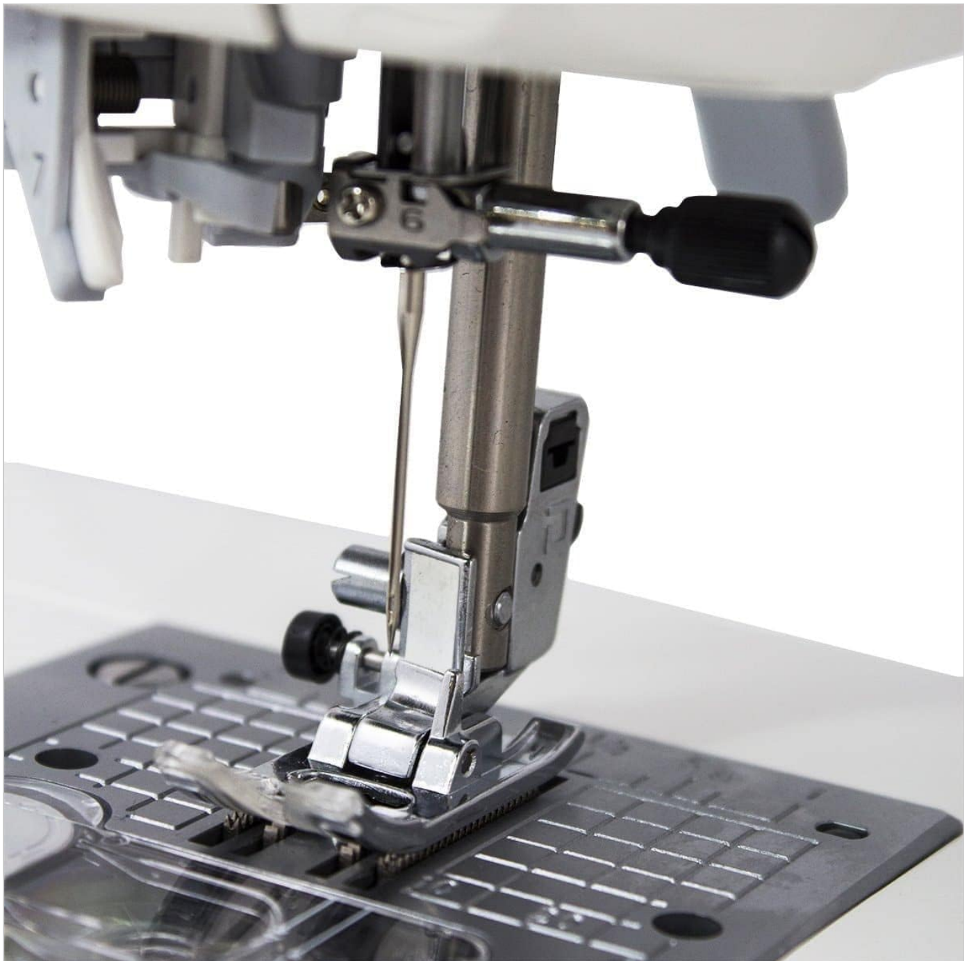
Figure 4.2: The Juki HZL-F400 with the upper thread correctly routed through the machine's guides and tension discs.
