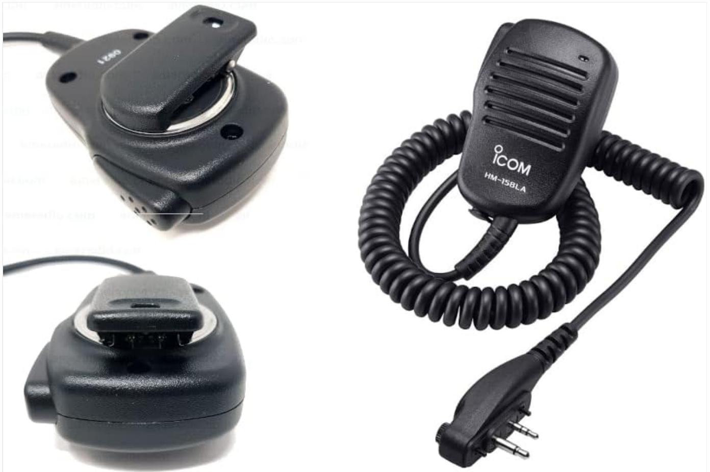
Figure 2: Multiple views of the Icom HM-158LA, illustrating the speaker microphone, coiled cable, 2-pin connector, and the rear view showing the alligator clip mechanism.
