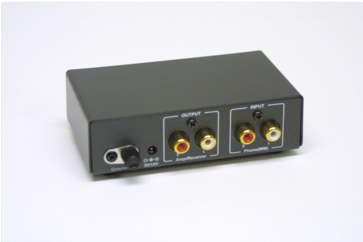
Figure 2: Rear view of the TEC TC-450 Mobile Phono Preamp. Displays the gold-plated RCA input (Phono MM) and output (Amp/Receiver) jacks, ground terminal, and DC12V power input.
