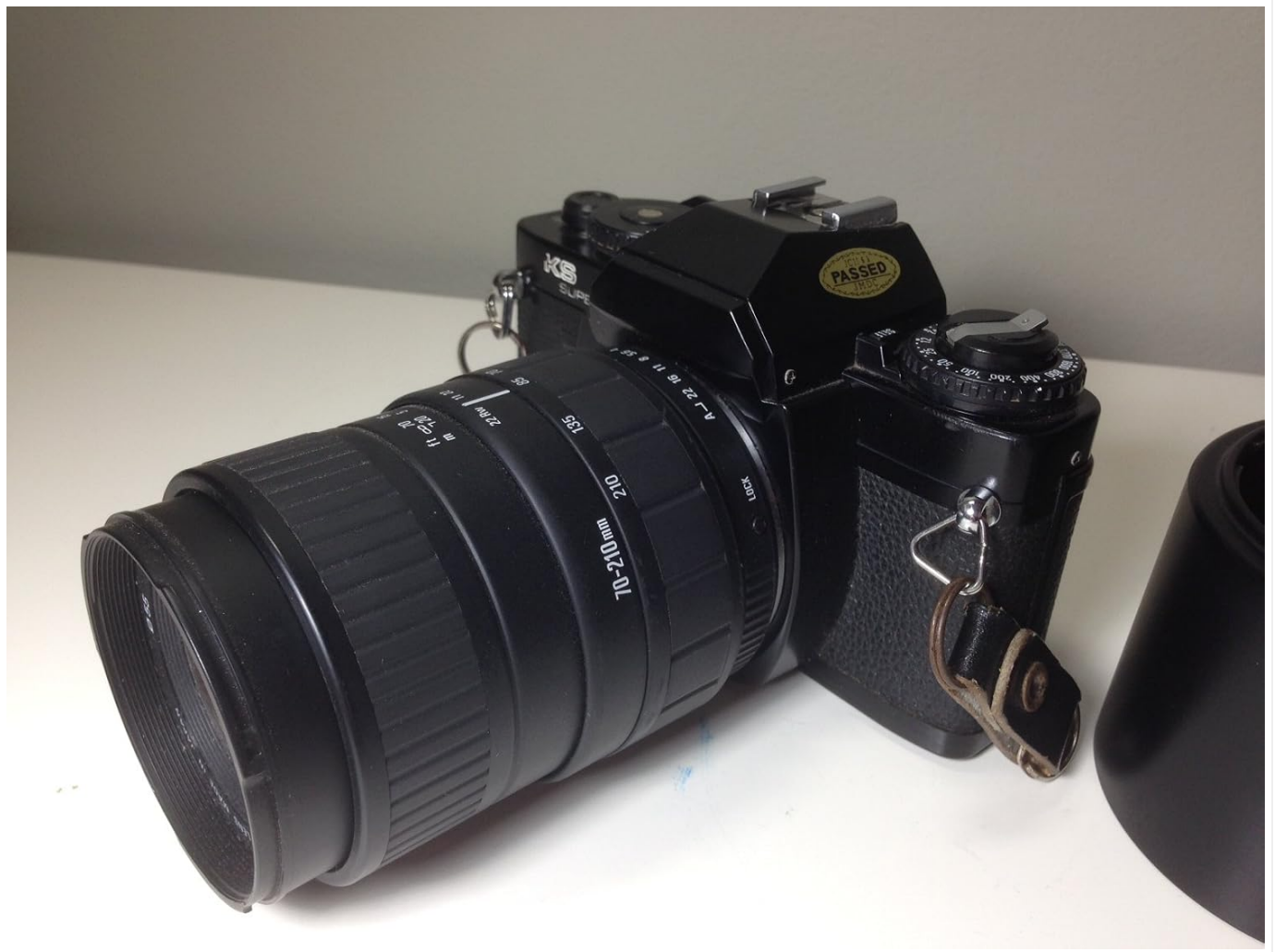
Figure 5: Side view of the camera with the Sigma Zoom 70-210mm lens, demonstrating the zoom extension.
