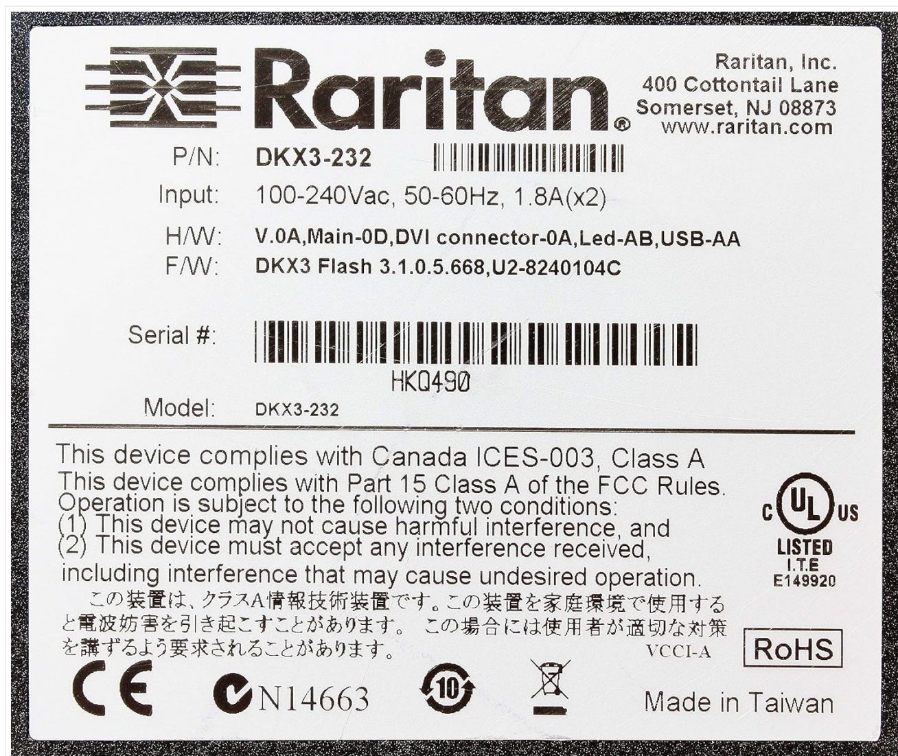
Figure 3: Product label for the Raritan Dominion KX III DKX3-232, displaying model number, serial number (HKQ490), input power specifications, and compliance markings (FCC, UL, CE, RoHS).
