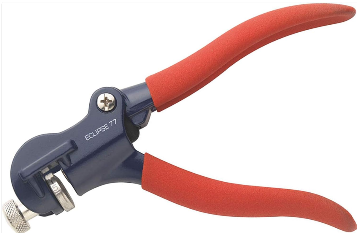
Figure 1: Overall view of the Spear & Jackson 94-370R Eclipse Saw Tooth Setter.
