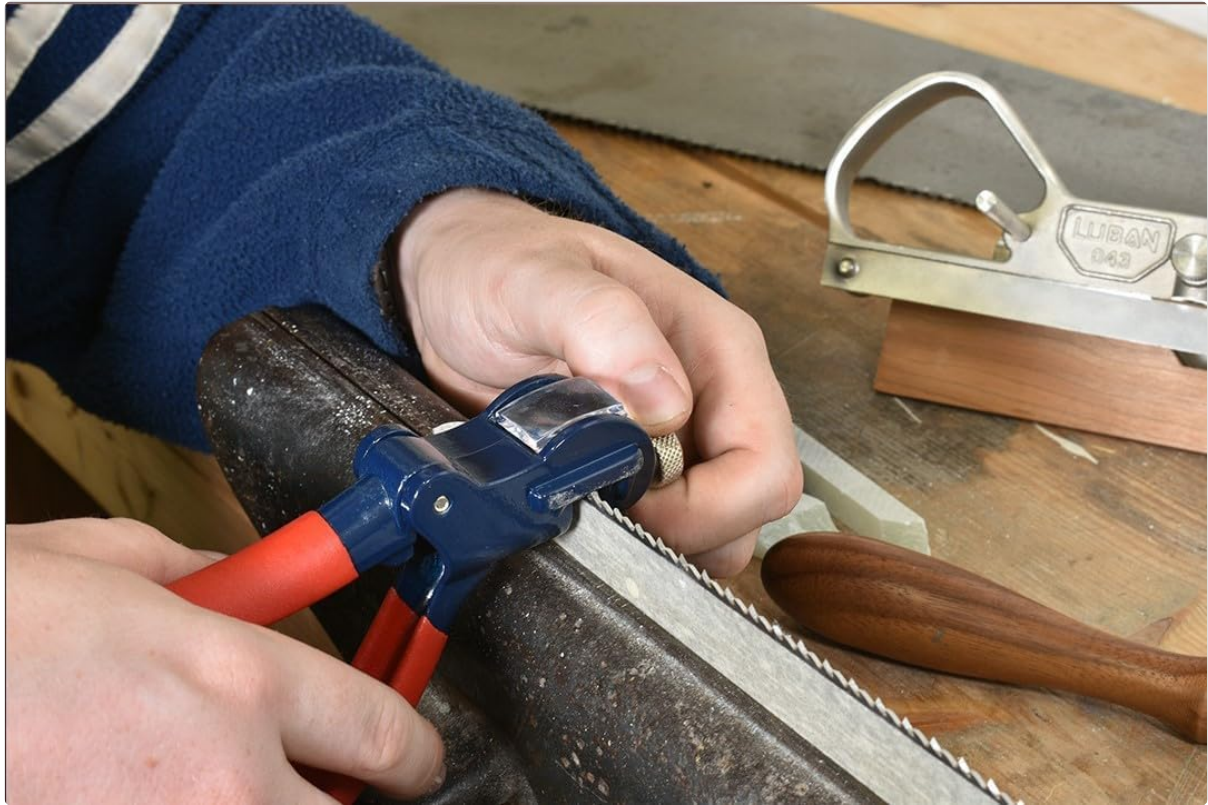
Figure 3: Demonstrating the saw tooth setter in use on a saw blade.
