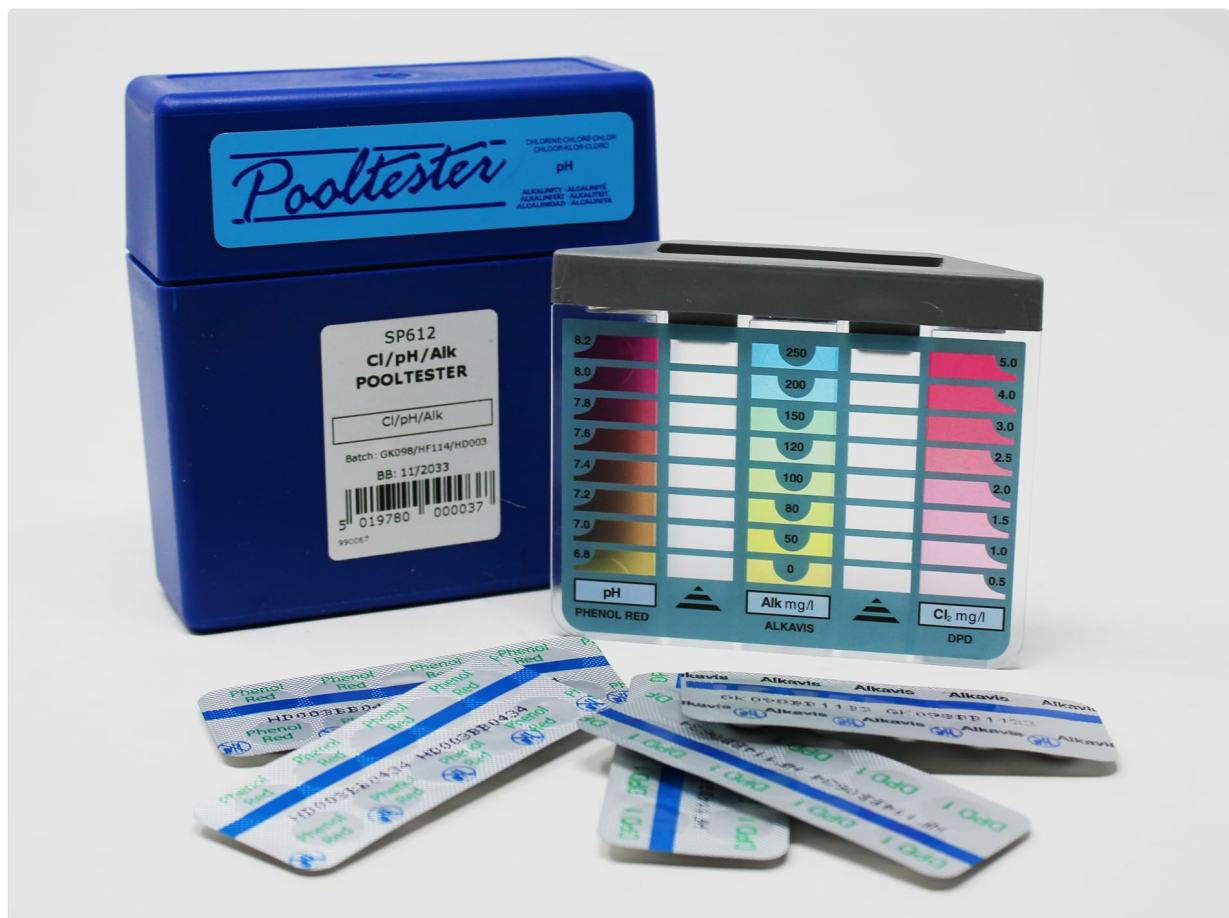
Figure 6.1: The Palintest color comparator block. This image shows the three scales for pH (Phenol Red), Alkalinity (ALK mg/l), and Chlorine (CL mg/l DPD), used to interpret test results.
