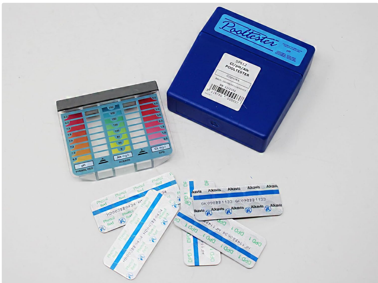
Figure 3.1: Overview of the Palintest SP 612 Pooltester Kit components. This image displays the blue Pooltester case, the color comparator block, and blister packs of DPD1, Phenol Red, and Alkavis tablets.
