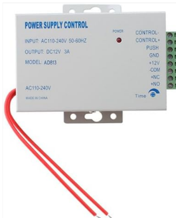
Figure 5.2: Power Supply Control Unit (AD813).
