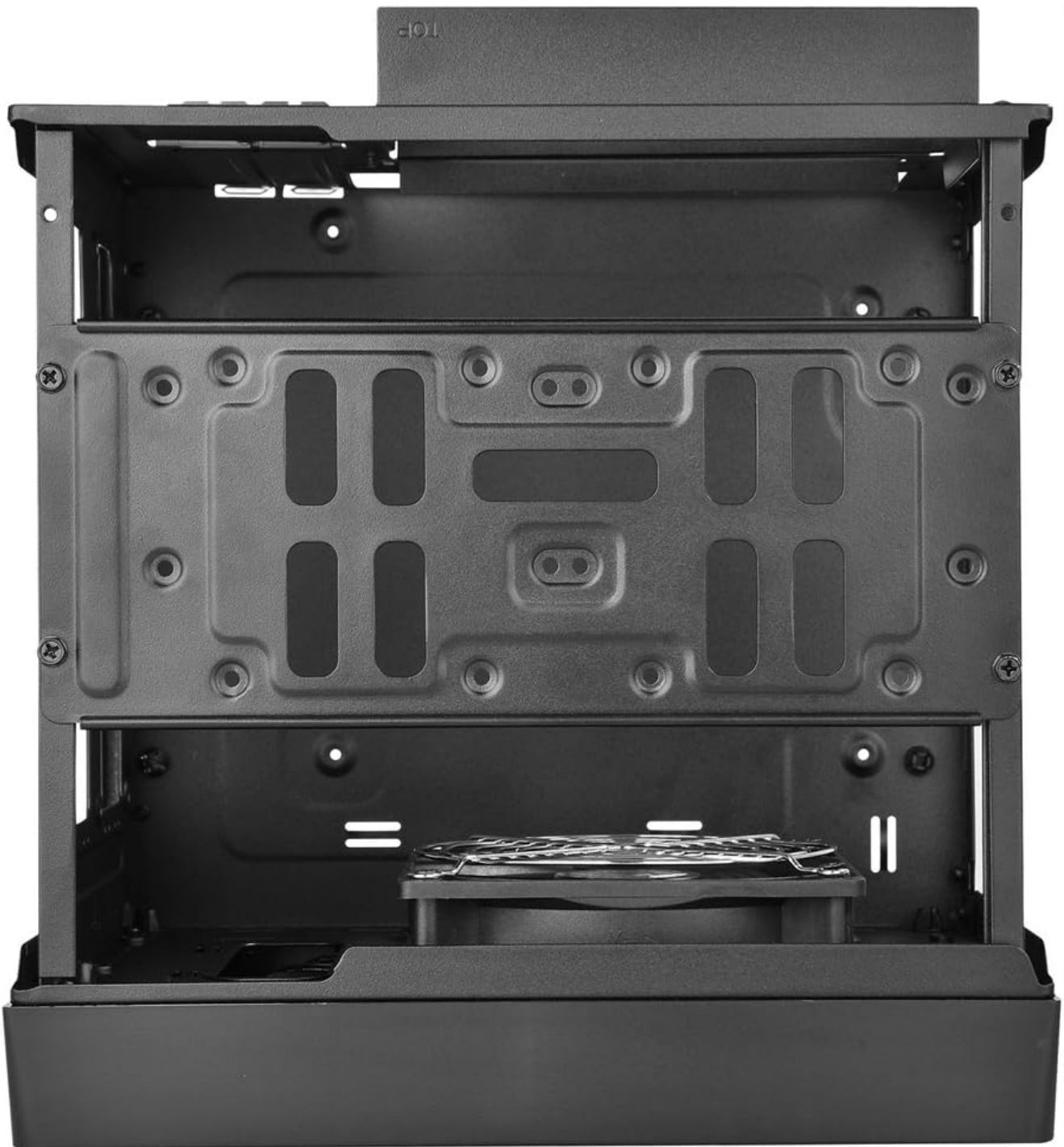
Figure 3.2: Internal view demonstrating the placement of a power supply unit and a Mini-ITX motherboard.
