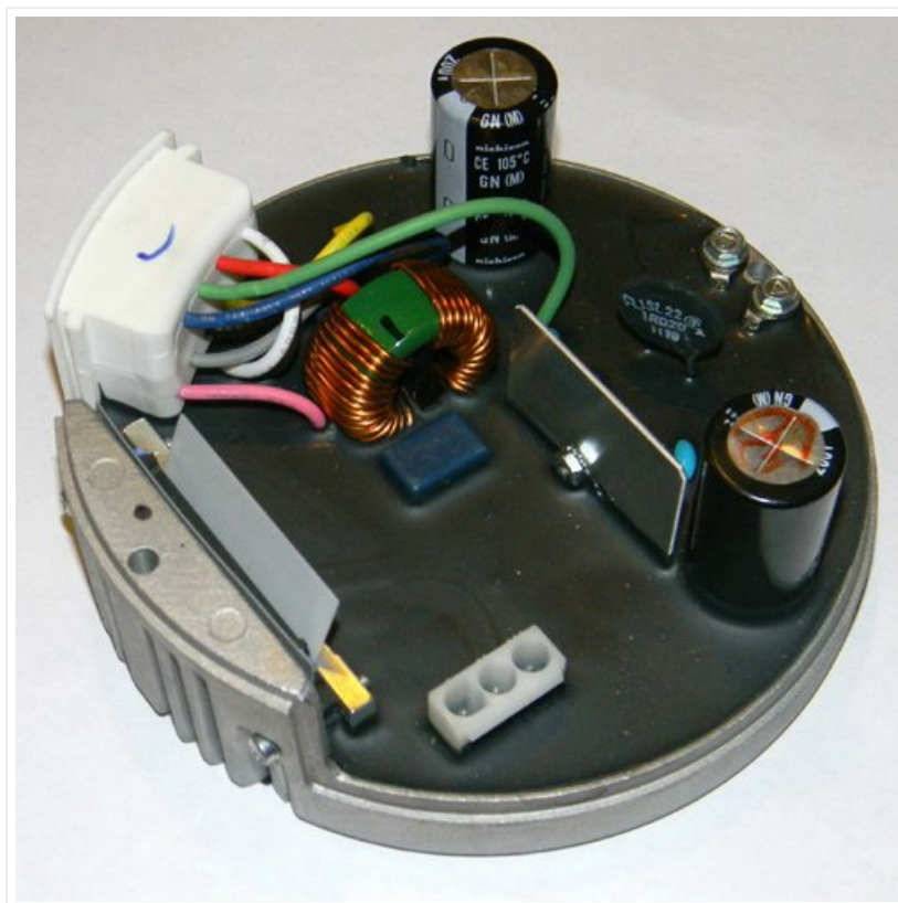
Figure 1: Top view of the Carrier HD52AE141 X13 Blower Motor Module, illustrating its internal electronic components, including capacitors, inductors, and the multi-colored wiring harness connector. The module features a robust design with a metal heat sink on one side.
