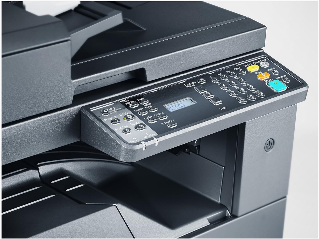
Figure 5.1: Detailed view of the control panel, showing buttons for print, copy, scan, and navigation.
