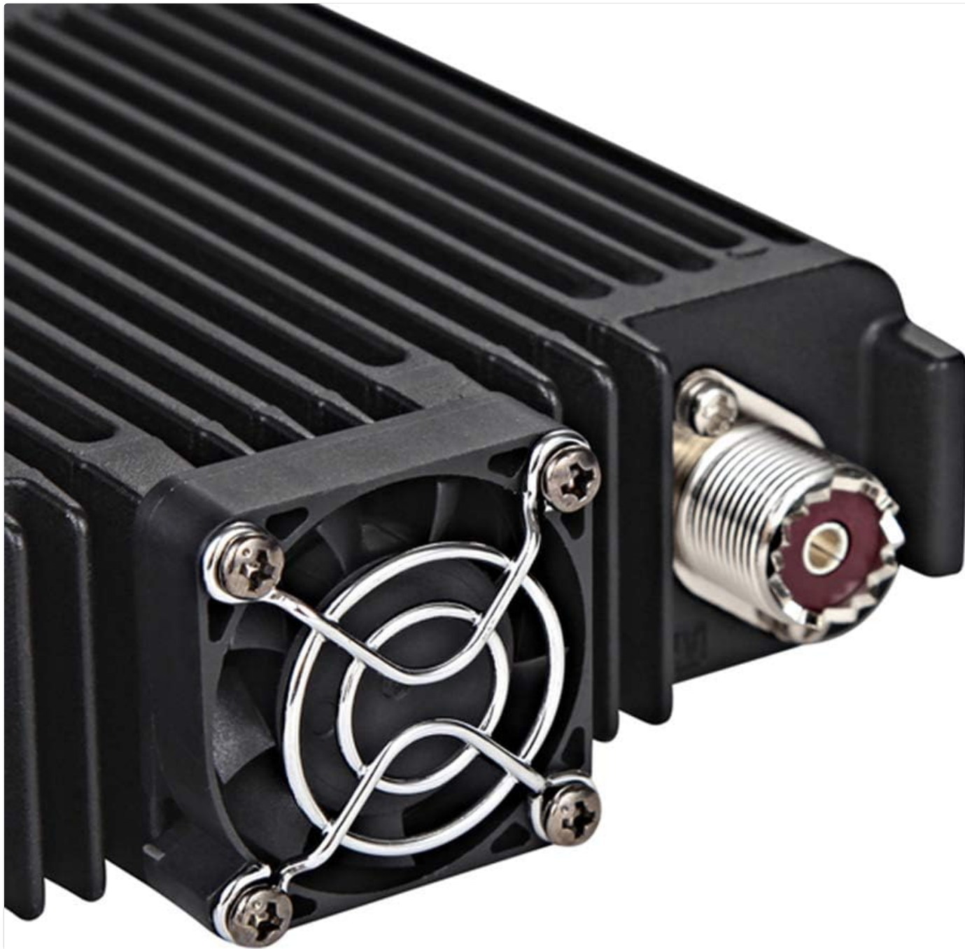
Figure 4.2.1: Close-up of the cooling fan and SO-239 antenna connector on the rear of the transceiver, emphasizing the importance of proper ventilation and antenna connection.
