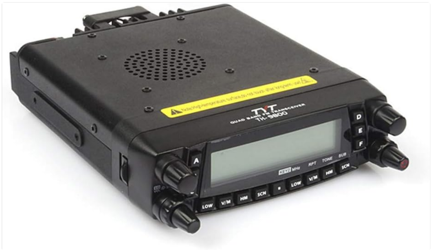
Figure 4.1.1: Side view of the TYT TH-9800 transceiver unit, showing its compact design suitable for mobile or fixed installations.
