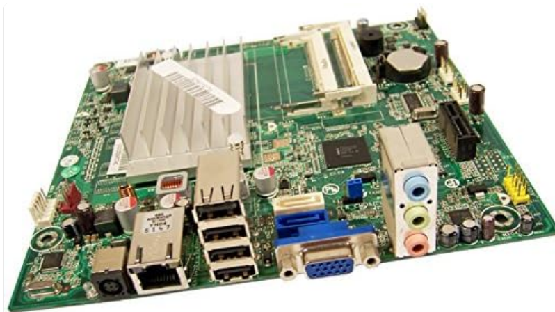
Figure 1: Overview of the Compaq 100eu All-in-One PC Motherboard (Model 619965-001). This image displays the various ports, slots, and components, including the CPU heatsink, RAM slots, SATA ports, USB ports, Ethernet port, and audio jacks.
