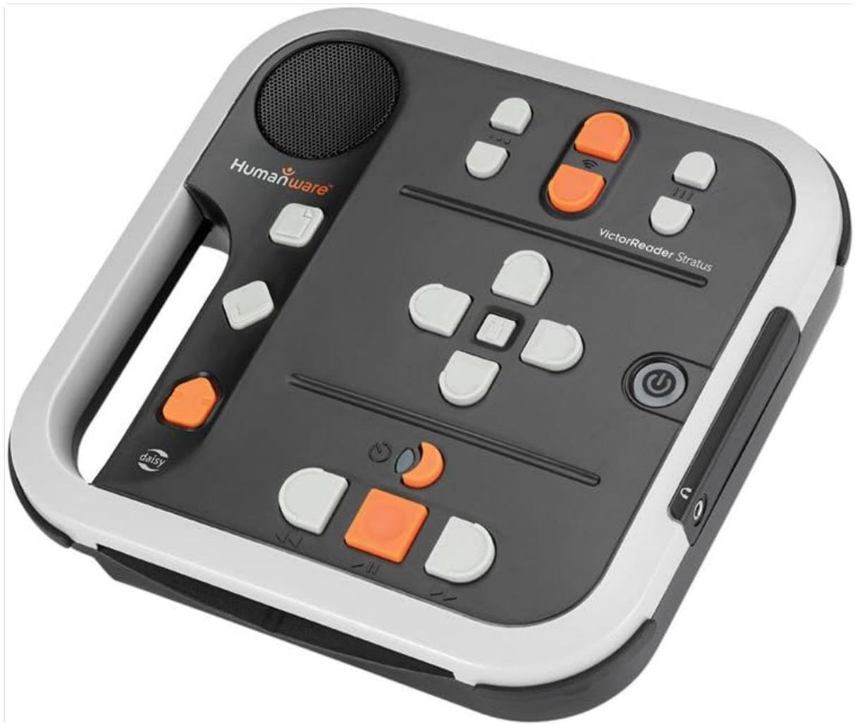
Figure 1: The HumanWare Victor Reader Stratus4 M, showcasing its intuitive button layout and integrated speaker.
