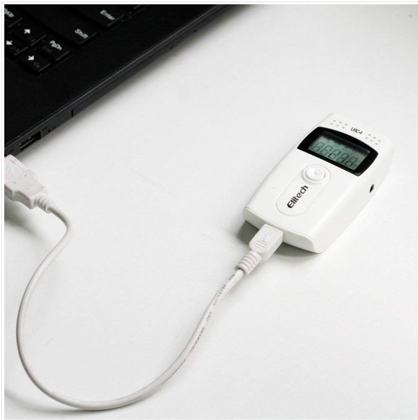
Figure 3: The Elitech RC-4 data logger connected to a computer via its USB port, ready for configuration or data download.
