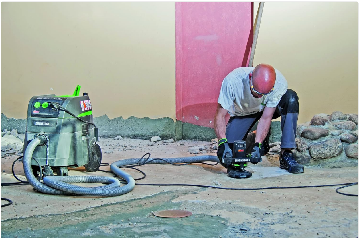
Figure 3: Industrial vacuum cleaner connected to a power tool for dust extraction.
