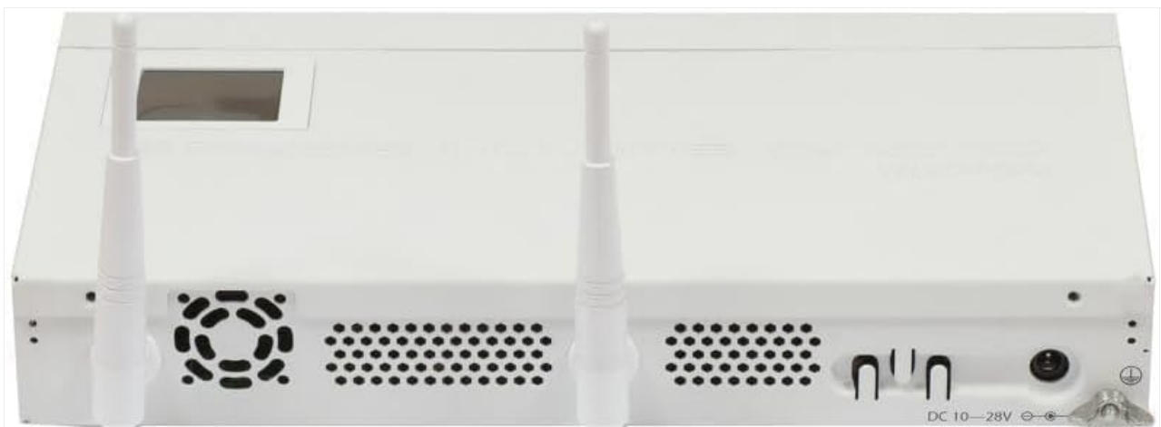
Figure 2: Rear view of the MikroTik CRS125-24G-1S-2HnD-IN device. This image shows the power input, grounding screw, and ventilation openings.
