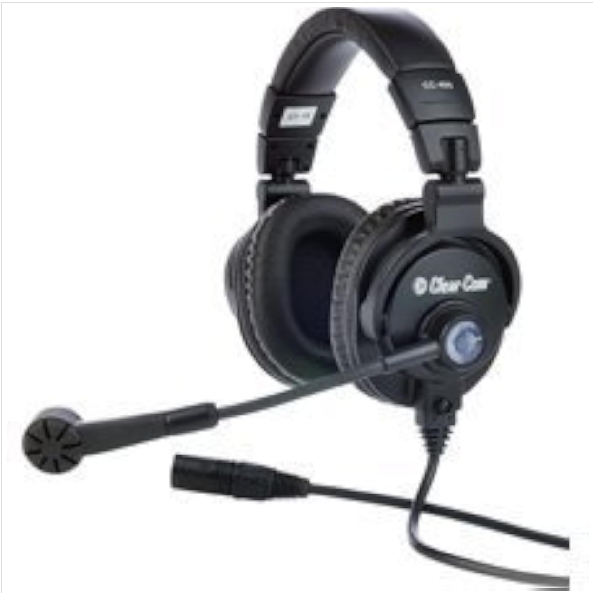
Image 2.1: Clear-Com CC-400-X4 Double-Ear Headset. This image displays the Clear-Com CC-400-X4 double-ear headset. It features large, circumaural earcups designed for noise attenuation, an adjustable headband, and a flexible microphone boom arm extending from the left earcup. The microphone is a hyper-cardioid dynamic type. A 4-pin female XLR connector is visible at the end of the headset cable.
