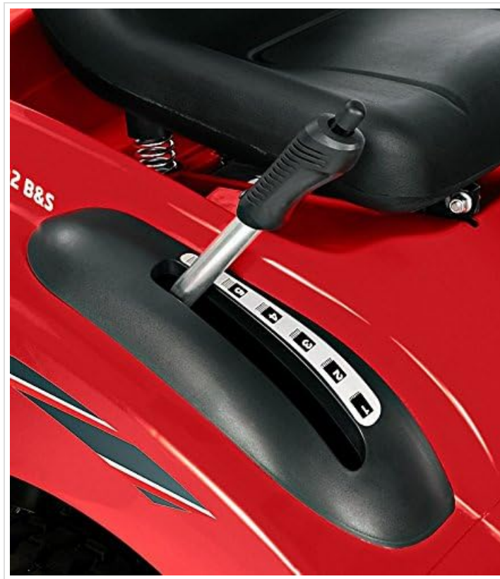
Image 2: Gear selector lever. This lever controls the forward and reverse speeds of the mower.
