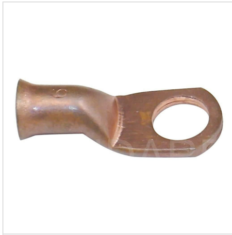
Figure 1: Standard Motor Products HP2800 Copper Battery Cable Lug. This image shows the copper lug with a cylindrical opening on one end for cable insertion and a flat, circular terminal on the other end for bolt connection. The lug is made of copper, indicating high conductivity.
