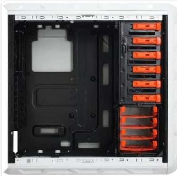
Figure 2: Detailed interior view showing the orange tool-less drive bay mechanisms for easy installation of storage devices.
