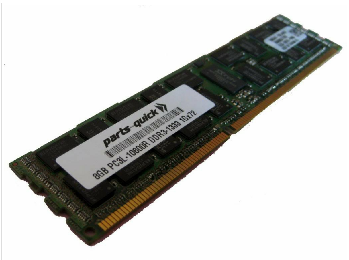
Figure 3.1: The parts-quick 8GB DDR3 PC3L-10600R 1333MHz ECC Registered Server DIMM RAM module. This image shows the physical appearance of the memory stick, including its chips and gold connector pins, ready for installation into a compatible server motherboard slot.
