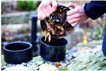
Image 4: Emptying the skimmer's debris collection basket.
