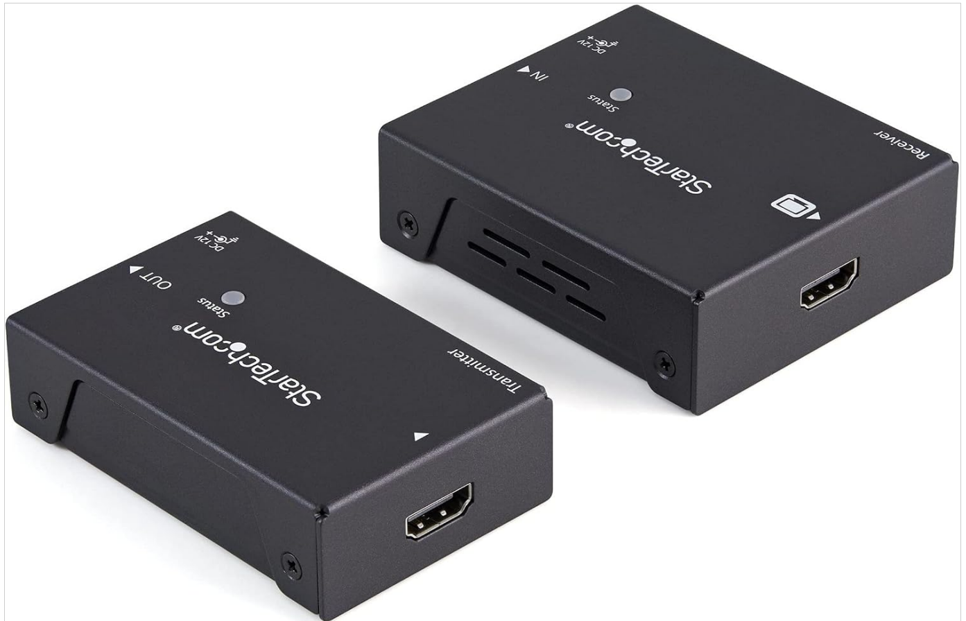
Image: The StarTech.com HDMI Extender Transmitter and Receiver units, showing their compact black enclosures and status indicators.
