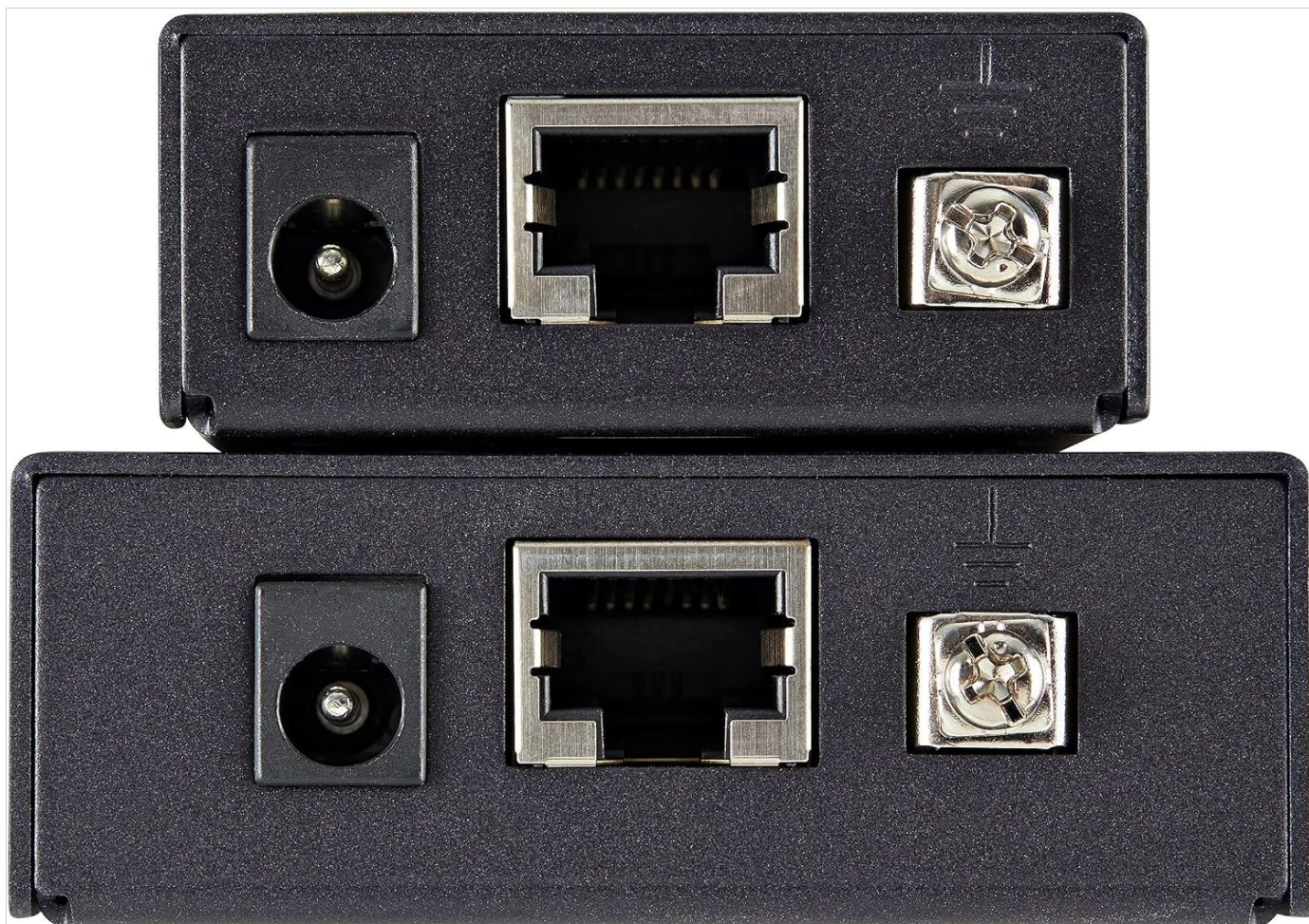
Image: A close-up view of the DC power input, RJ45 Ethernet port, and grounding screw on the StarTech.com HDMI Extender units.
