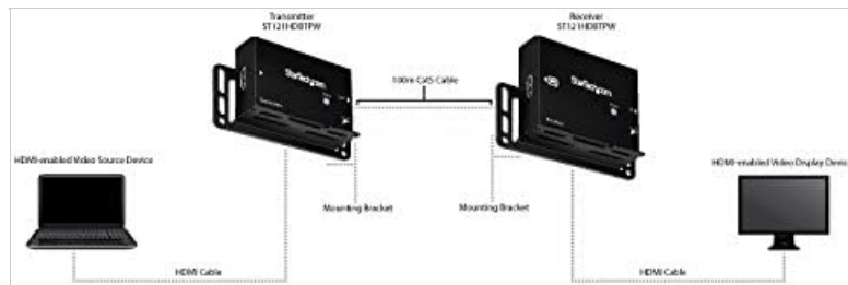
Image: A connection diagram illustrating how to connect the HDMI-enabled video source to the Transmitter (ST121HDBTPW), the Transmitter to the Receiver (ST121HDBTPW) via a 100m CAT cable, and the Receiver to the HDMI-enabled video display device. Mounting brackets are also shown.
