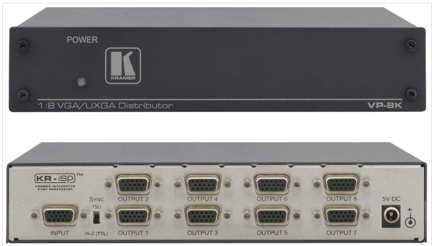
Figure 1: Front and Rear Panels of the Kramer VP-8K Distribution Amplifier. The top view shows the front panel with the "POWER" indicator and "1:8 VGA/UXGA Distributor" label. The bottom view displays the rear panel with one VGA/UXGA input, eight VGA/UXGA outputs, a sync impedance switch, and the 5V DC power input.
