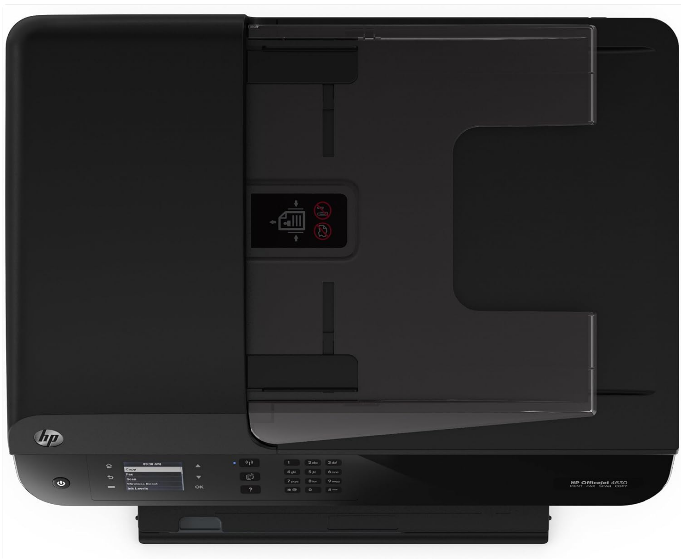
Figure 4: Top view of the HP Officejet 4630 e-AiO, highlighting the Automatic Document Feeder for multi-page scanning and copying.
