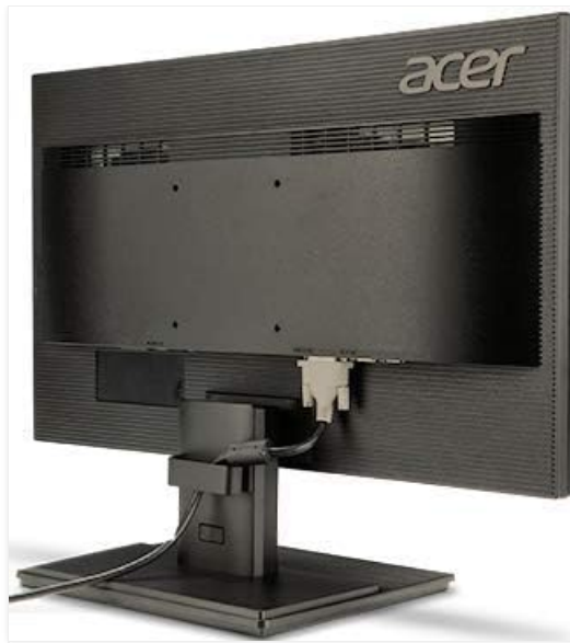
Figure 2.2.1: Rear view of the Acer V246HL monitor showing the stand attachment point and input ports. A VGA cable is shown connected.
