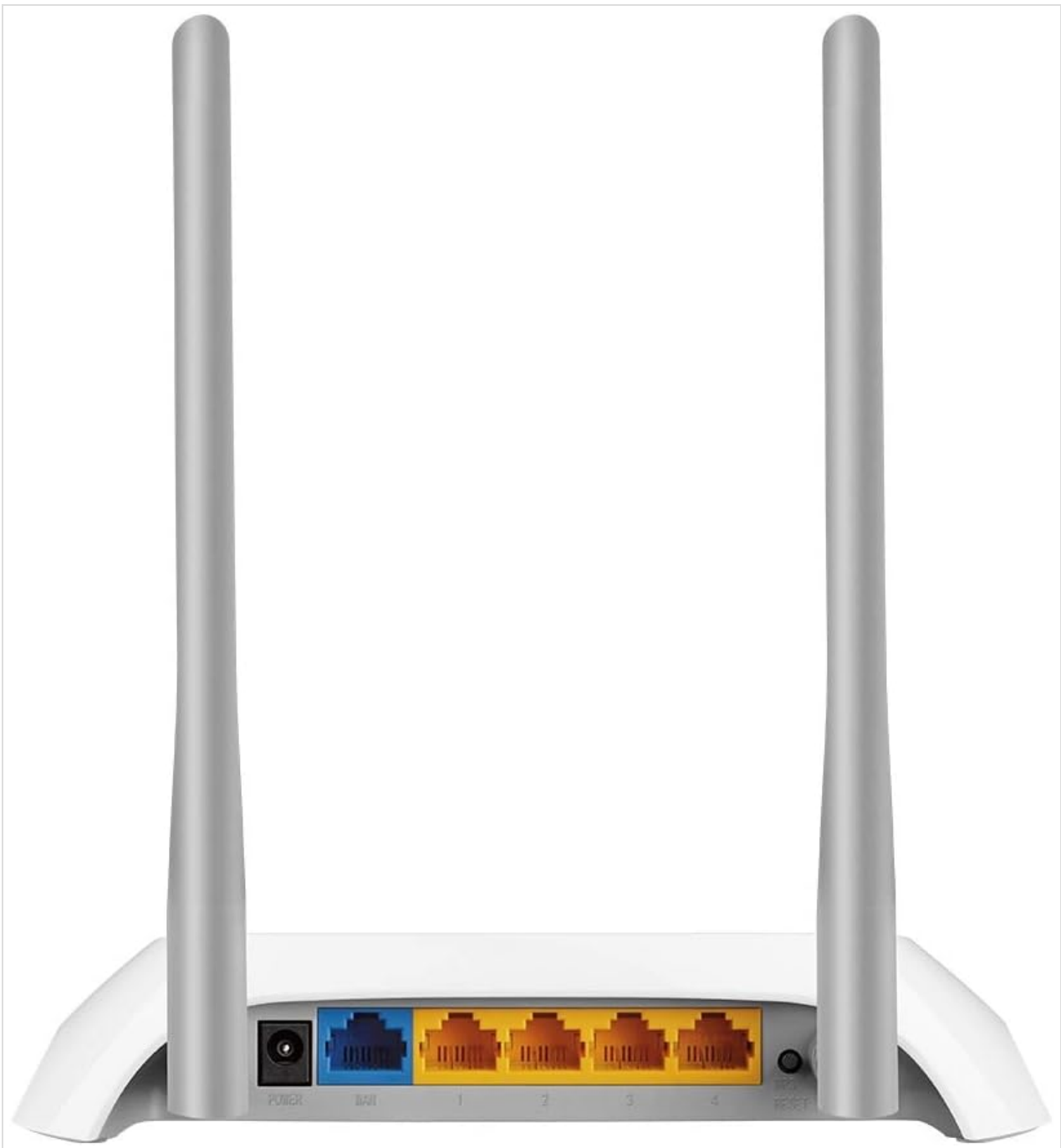
Image 2.2: Rear view of the TP-Link TL-WR840N Router, detailing the power input, blue WAN port, four yellow LAN ports, and the WPS/Reset button.
