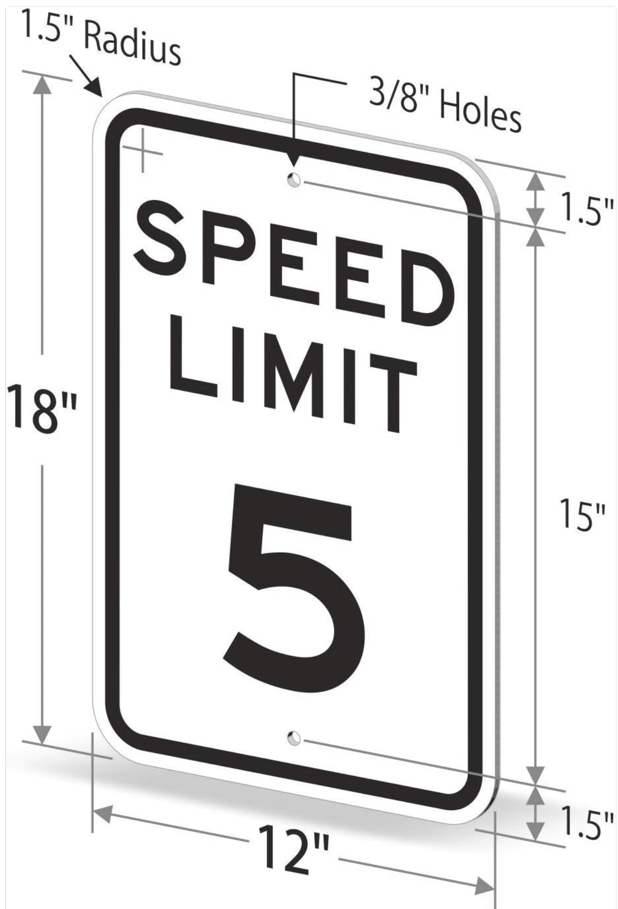
Figure 4: Dimensional diagram of the sign, indicating 12" x 18" size and 3/8" pre-drilled holes for mounting.
