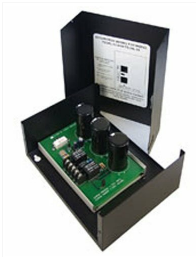
Figure 1: Securitron FSUNL-12 UnLatch Strike module. This image shows the electronic circuit board with capacitors and relays housed within a black metal enclosure. A white label with product information is visible on the inside of the enclosure's lid.
