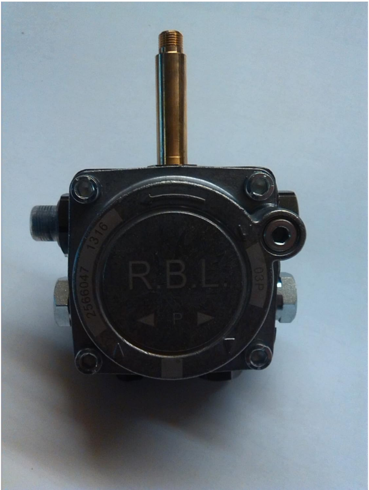
Figure 1: Riello Oil Pump Model 3007771. This image shows the overall structure of the oil pump, including the shaft, mounting points, and connection ports. The pressure adjustment screw is visible on the front face, marked with 'R.B.L.' and directional arrows.
