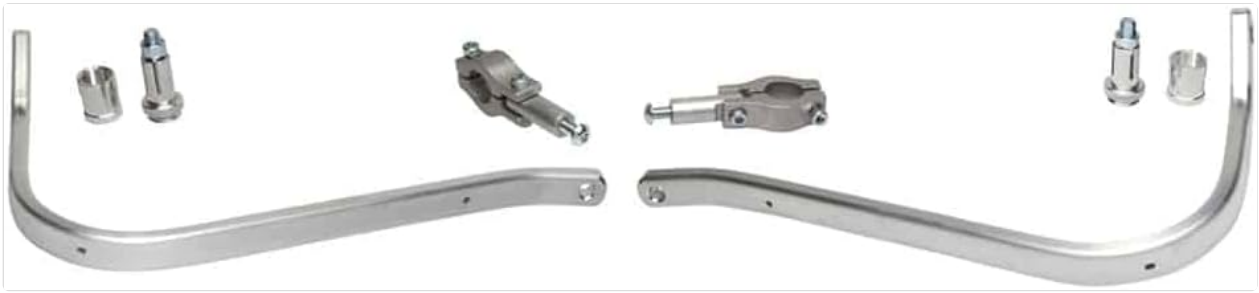
Figure 1: Complete Barkbusters VPS Black Handguard kit showing all components.
