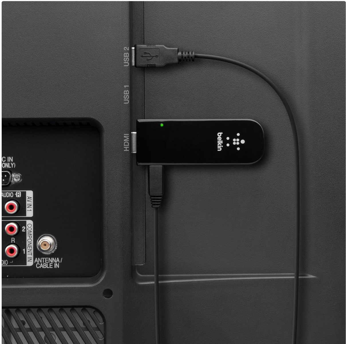
Image: The Belkin Miracast Video Adapter connected to an HDTV's HDMI port and receiving power from a USB port on the TV.
