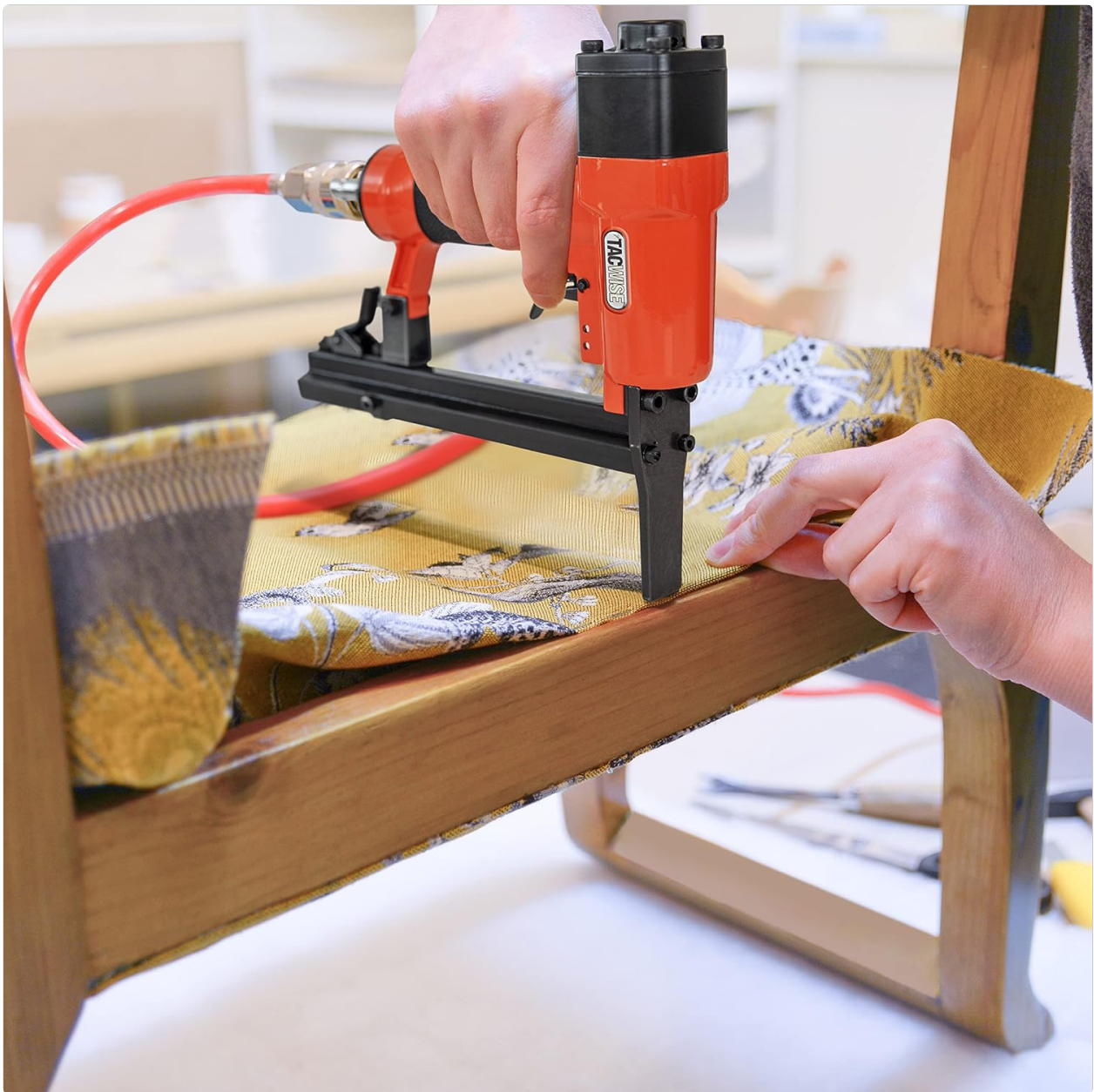
Figure 5: Applying staples to a chair during upholstery.
