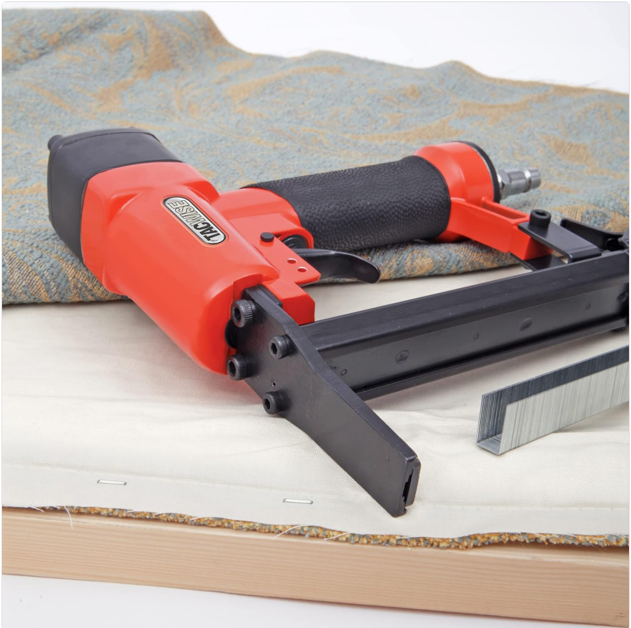
Figure 6: Use of correct Type 80 staples is essential for proper function.
