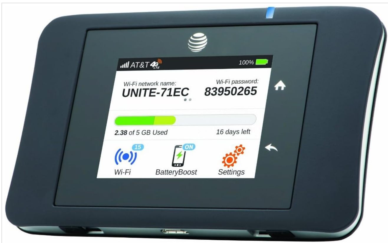
Image: Front view of the NETGEAR Unite Pro Hotspot, showing the touchscreen display with network information.
