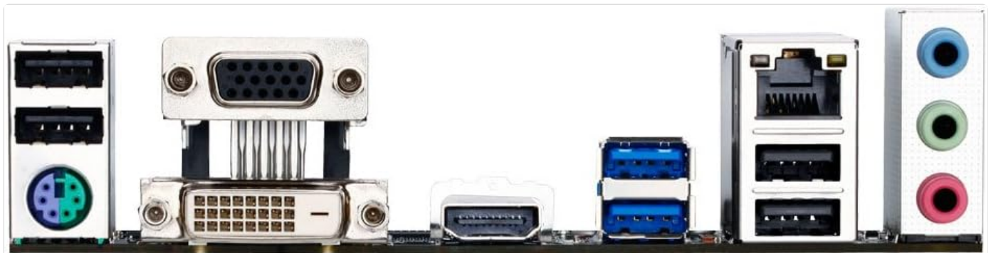
Figure 4.4: Close-up view of the rear I/O panel, showing ports for PS/2, D-SUB, DVI-D, HDMI, USB 3.0/2.0, LAN, and audio jacks.
