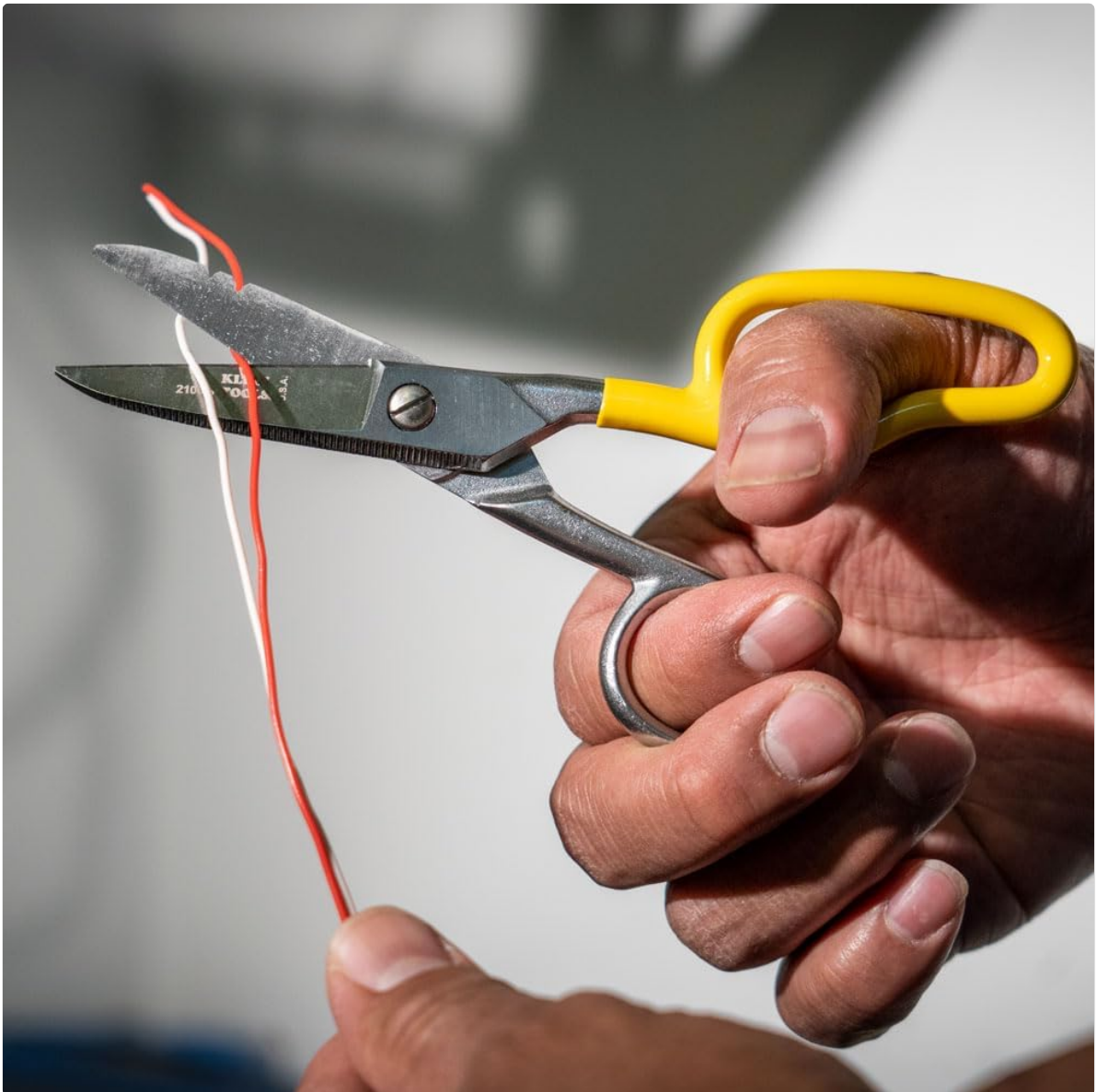
Image 4.1: Demonstrating the wire stripping function of the snips.
