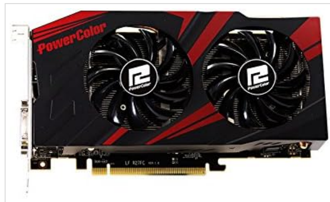
Figure 2.2.2: Front view of the PowerColor TurboDuo R9 270X Graphics Card, highlighting the dual cooling fans and PowerColor branding.
