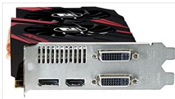
Figure 2.2.3: Close-up view of the PowerColor TurboDuo R9 270X Graphics Card's display output ports, including DVI, HDMI, and DisplayPort.
