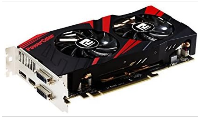
Figure 2.2.1: Angled view of the PowerColor TurboDuo R9 270X Graphics Card, showing its dual-fan cooler and display outputs.
