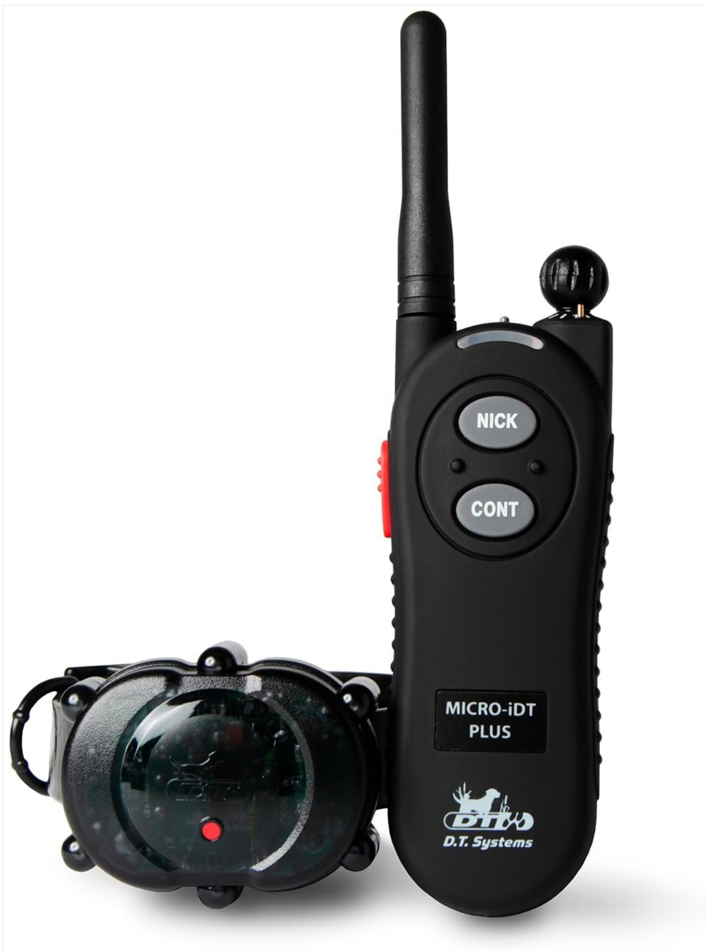
Image: The Micro-iDT Plus system, showing the handheld transmitter and the dog collar receiver.
