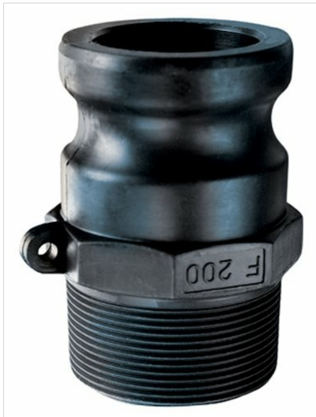
Figure 1: A black polypropylene Part F male adapter with a cam and groove connection on one end and a male NPT threaded connection on the other. The NPT threads are visible at the bottom, and the cam and groove portion is at the top. The fitting is marked 'F 200'.
