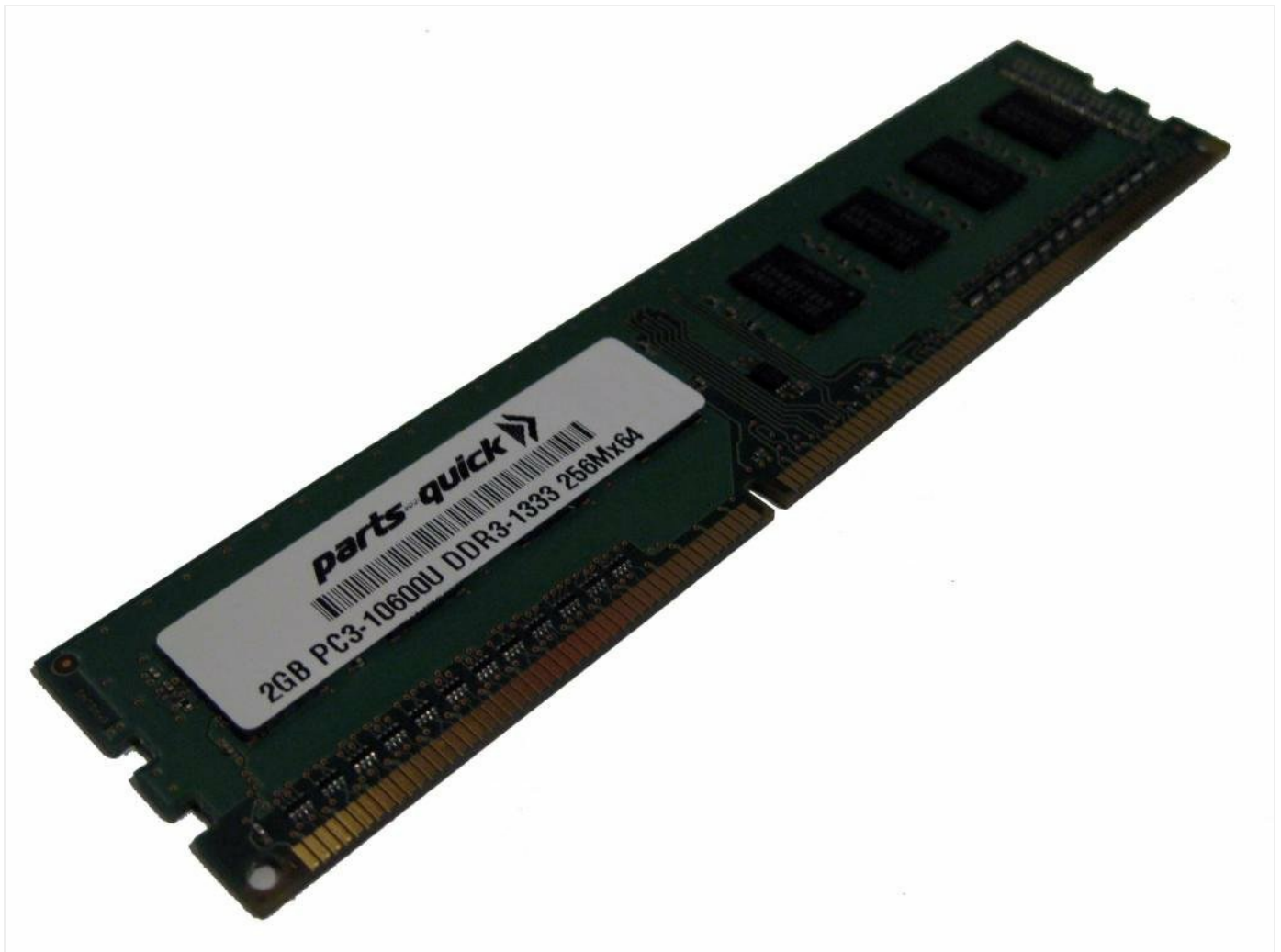
Image: The parts-quick 2GB DDR3 1333 MHz DIMM memory module. This image shows the physical appearance of the RAM stick, including its chips and gold contacts.
