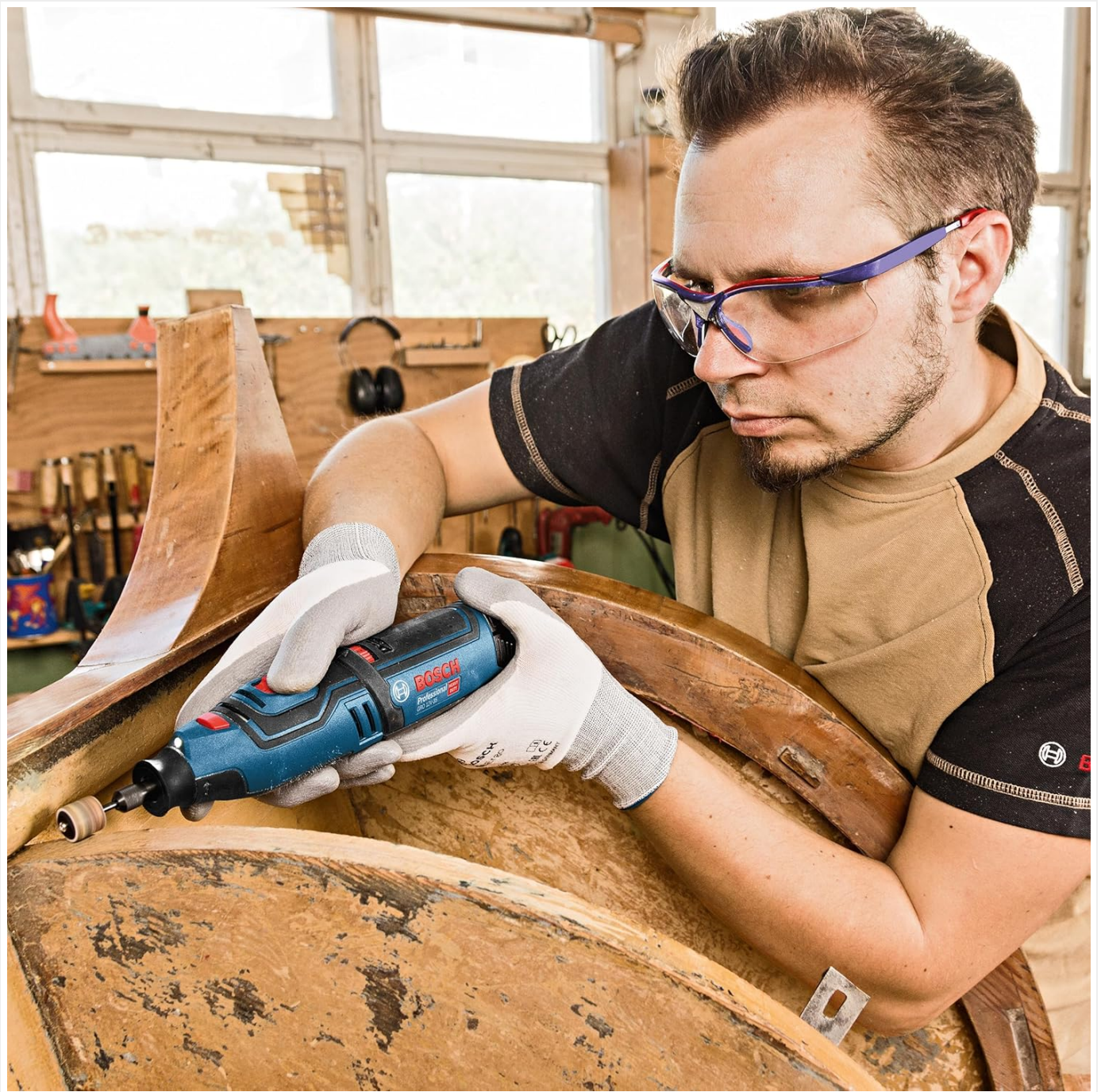
Figure 4.2: Sanding a wooden surface with the rotary tool. Maintain a firm grip and control.
