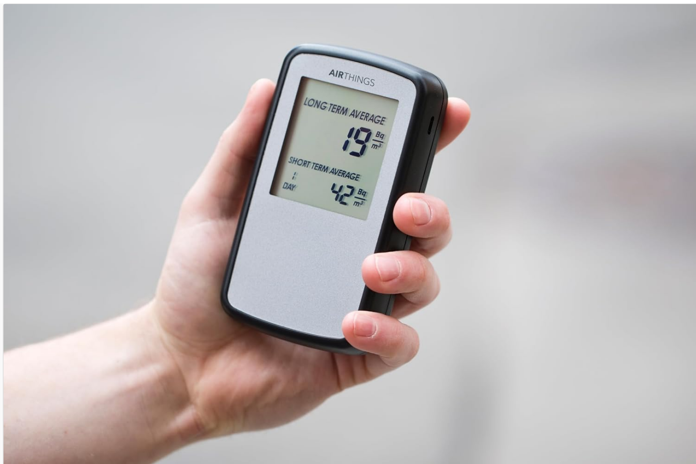
Figure 2.1: The AIRTHINGS Corentium Home detector in hand, displaying radon levels.
