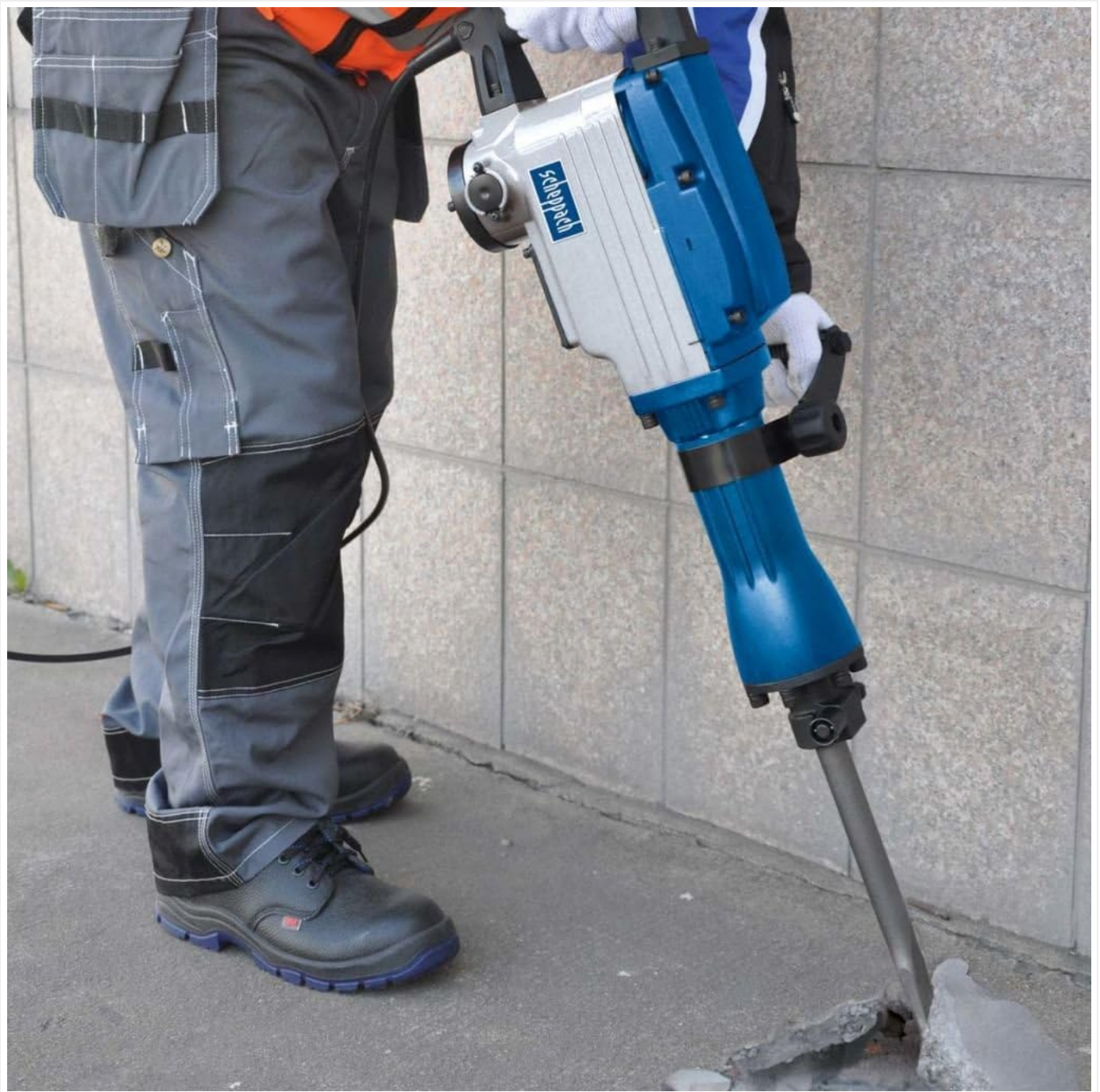
Figure 5: An operator demonstrating the use of the Scheppach AB1600 to break concrete, highlighting the tool's ergonomic design for effective downward force.
